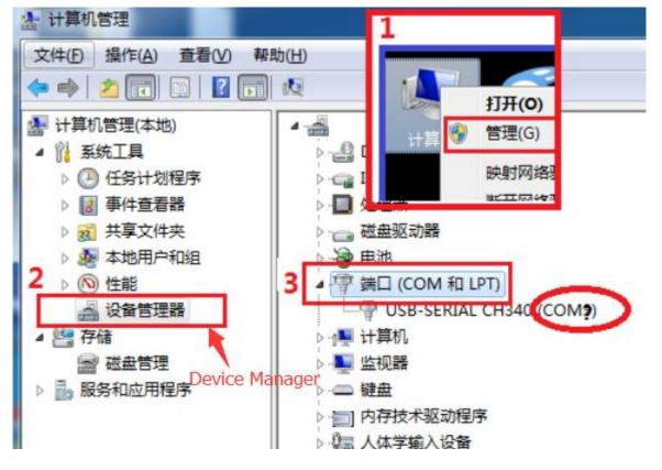
• Open grblControl software to connect the machine, choose the correct port:
